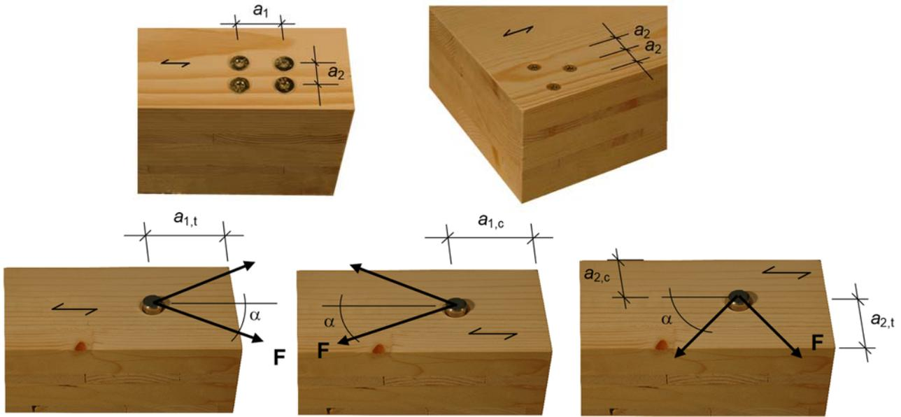
Definition of spacing, end and edge distances in the edge surface unless otherwise specified in the technical specification (ETA or hEN) for the cross laminated timber:
