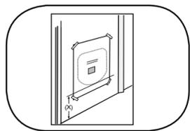
Position the template base at belly height marked on door (X).
