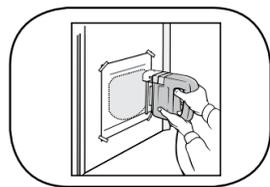
Using a jig or key-hole saw cut along the cutting circle as indicated.
